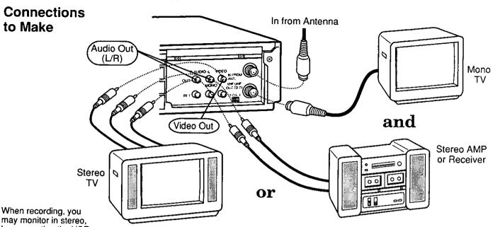
by connecting the VCR to either a stereo TV, or a mono sound TV with an external stereo amp and speakers.
